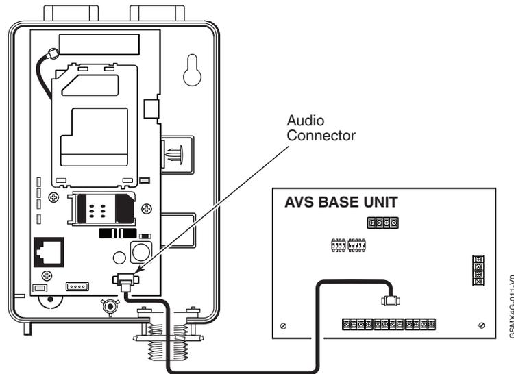
2. Connect one end of the audio cable (5-pin connector) to the audio connector located on the PC board in the communicator.
